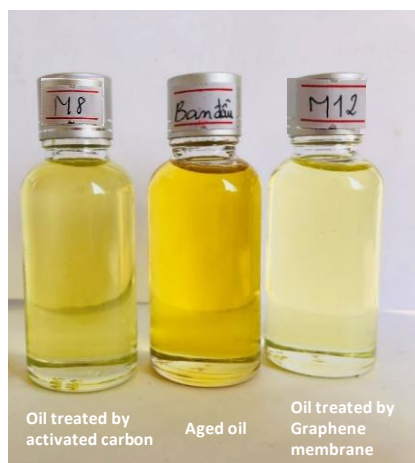
Figure 5: The colour of the aged oil, oil treated by activated carbon and Graphene membrane
