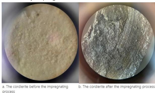
Figure 1: The magnification image of the CuMnO<sub>x</sub> supported on cordierite
