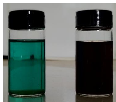
Figure 1: The color change of solution during the reduction of Cu 2+ to Cu + and Cu 0
