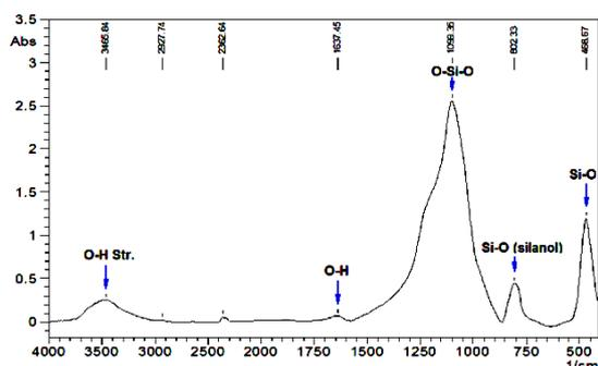
Figure 4: FT-IR spectrum of silica nanoparticles from industrial waste RHA
