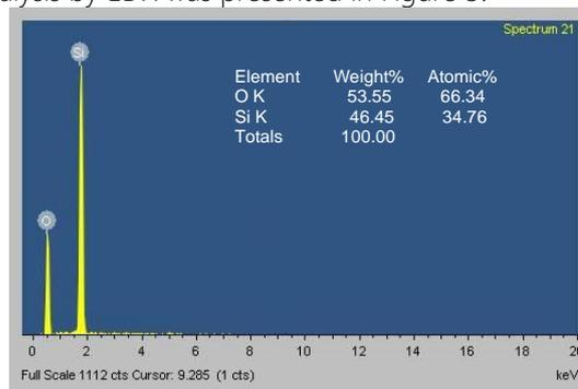
Figure 3: EDX spectrometric data of silica nanoparticles produced from RHA
