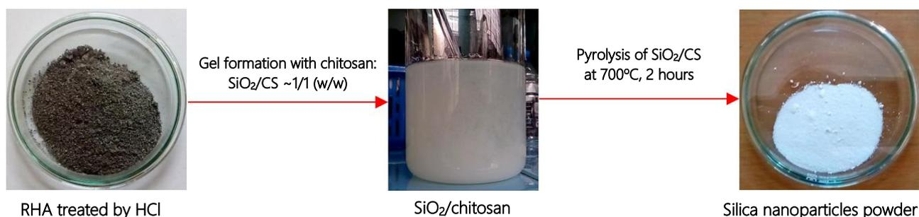
Figure 1: Simulation of the preparation process of silica nanoparticles by SiO<sub>2</sub>/chitosan gel pyrolysis
