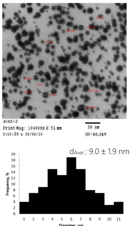
Figure 2: TEM images and distribution of particle size of silica nanoparticles from industrial waste RHA
