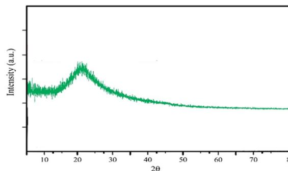
Figure 5: XRD pattern of silica nanoparticles from industrial waste RHA
