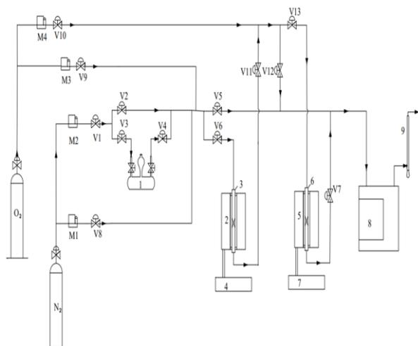
Figure 1: Schematic diagram of toluene Oxidation experiment
