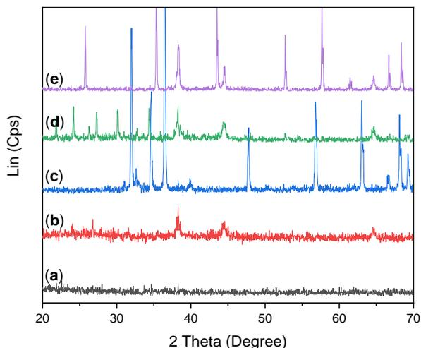
Figure 1: XRD patterns of a) Ag-Bent; b) Ag-C; c) Ag-ZnO; d) Ag-Zeolit; e) Ag-Al<sub>2</sub>O<sub>3</sub>
