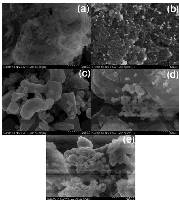
Figure 3: SEM image of a) Ag-Bent; b) Ag-C; c) Ag-ZnO; d) Ag-Zeolit; e) Ag-Al<sub>2</sub>O<sub>3</sub>
