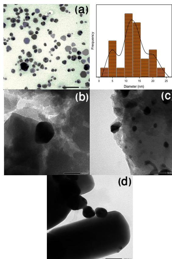
Figure 2: TEM image of a) Ag nanoparticles; b) Ag-Al<sub>2</sub>O<sub>3</sub>; c) Ag-C; d) Ag-ZnO
