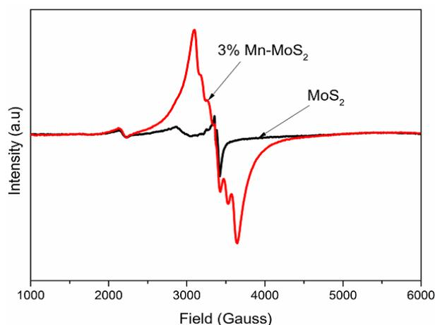
Fig 5: EPR spectroscopy of MoS<sub>2</sub> and 3%Mn-MoS<sub>2</sub>
