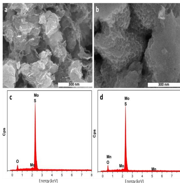
Fig 4: SEM images of  $\text{MoS}_2$  (a) and  $3\%\text{Mn-MoS}_2$  (b); EDX spectra of  $\text{MoS}_2$  (c) and  $3\%\text{Mn-MoS}_2$  (d)
