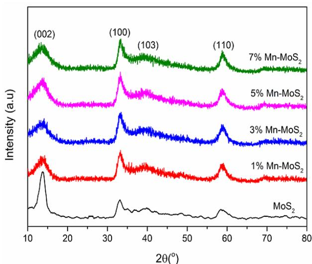
Fig 1: Effect of Mn content on crystal phase characteristics of Mn-doped samples (n% Mn-MoS<sub>2</sub>, with n = 1% Mn, 3% Mn, 5% Mn and 7% Mn)
